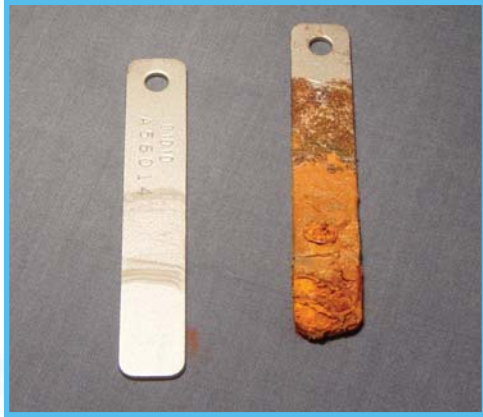
The corrosion coupon (right) was installed in an untreated hot water loop for 30 days. The coupon on the left was installed in a treated hot water loop for the same period.
